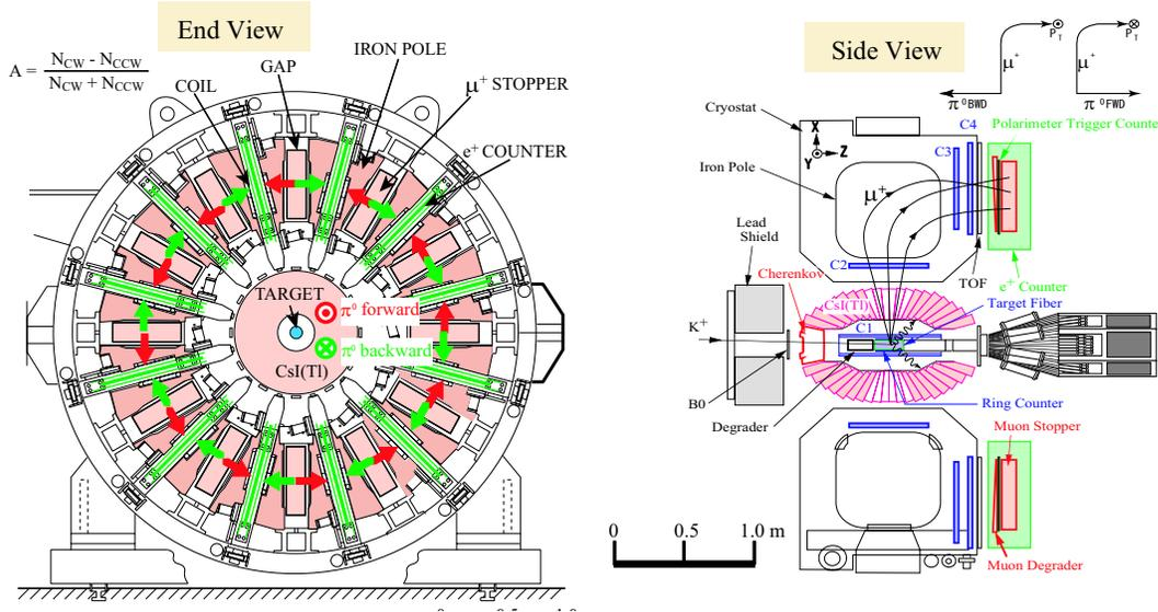
**Figure 1:** Experimental setup of the KEK-PS E246 experiment: (a) cross section side view and (b) end view. The E246 experiment employed the stopped  $K^+$  beam in conjunction with a superconducting Toroidal spectrometer. The detector system consisted of a large-acceptance CsI(Tl) barrel, tracking chambers, an active  $K^+$  target, and passive muon polarimeters. See [2] for details.
