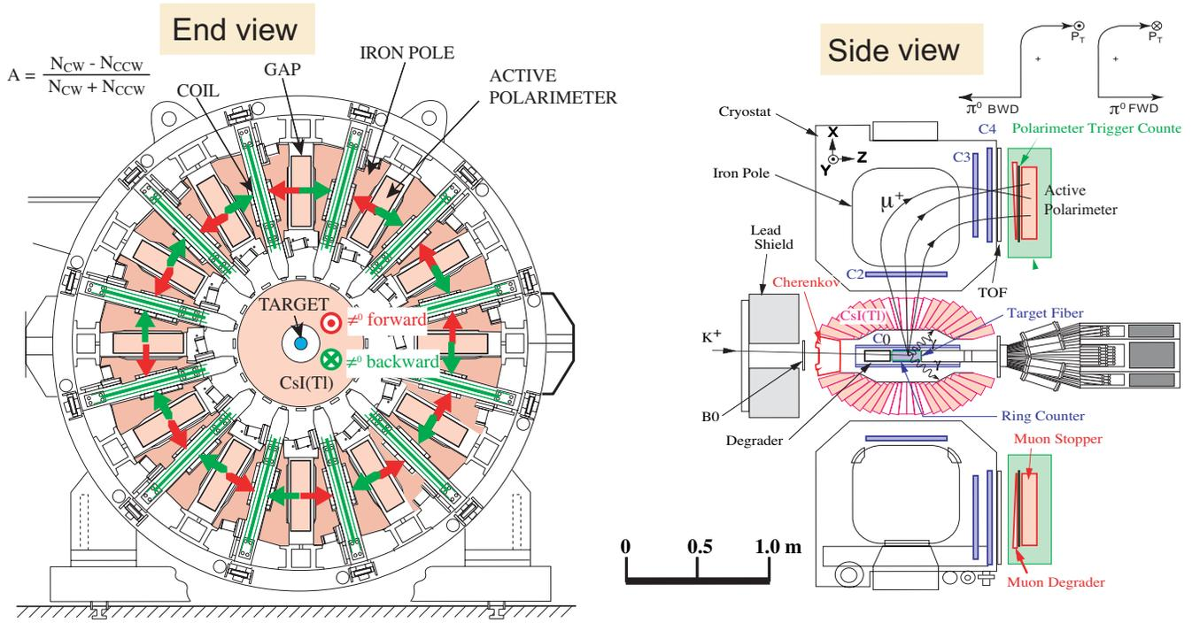
Fig. 2. TREK experimental setup with the Superconducting Toroidal Spectrometer.
