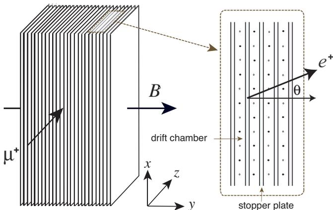
Fig. 3. Schematic view of the active muon polarimeter for one sector. Muons are stopped in the stopper plates. The field strength of  $B$  is 0.03 T.
