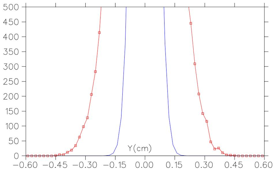
Figure 3: The vertical beam spot at IFY for the 0.8 GeV/c beam from the higher order Monte Carlo calculation with ZGOUBI. The blue curve is the input gaussian with  $\sigma$  of 1.3 mm times the magnification of 0.35
