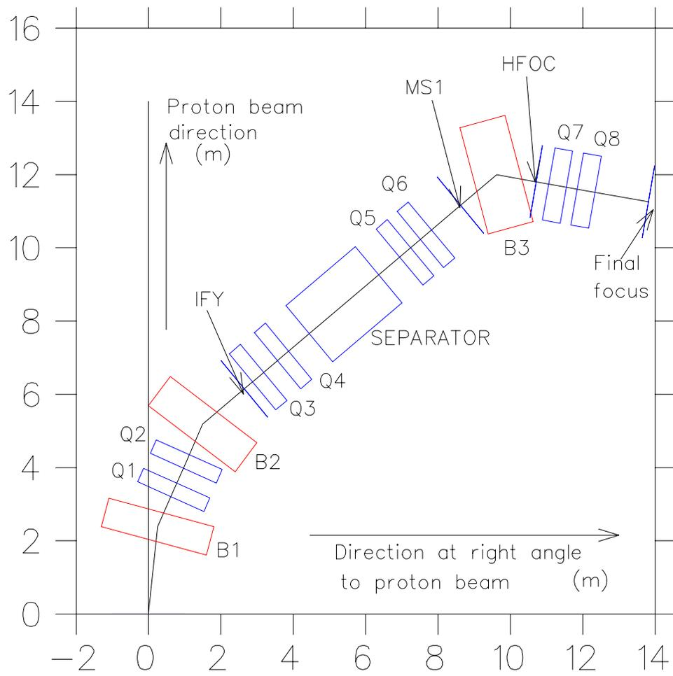
Figure 1: Layout of the 0.8 GeV/c beam.
