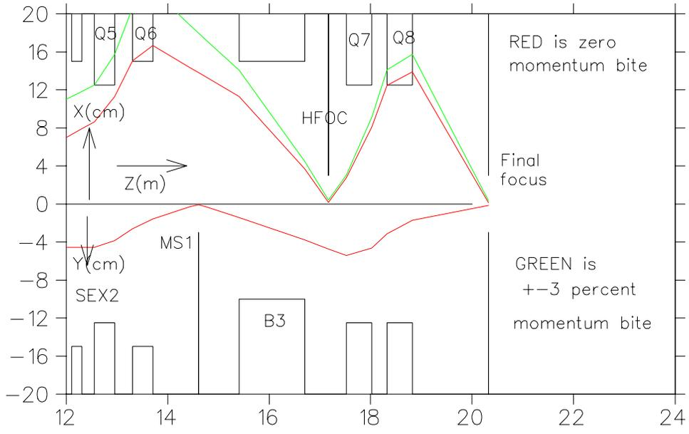
Figure 2: First order beam envelopes from TRANSPORT. The initial horizontal angle is 35 mr, the vertical angle is 9 mr. X is 3.5 mm and Y is 2 mm. All numbers indicate half widths. Red is for the central momentum. Green is for 3 percent  $\Delta P/P$
